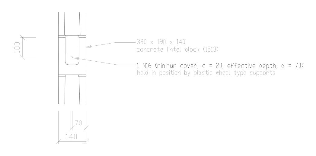
Reinforced Concrete Masonry Bond Beam Manafactured By Island Block & Paving
