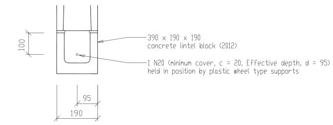
Reinforced Concrete Masonry Lintel Manafactured By Island Block & Paving Scale 1:10
