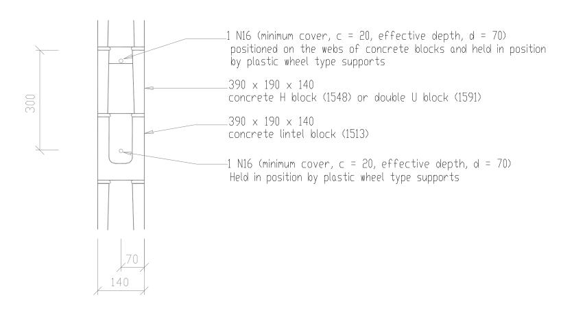
Reinforced Concrete Masonry Bond Beam Manafactured By Island Block & Paving
