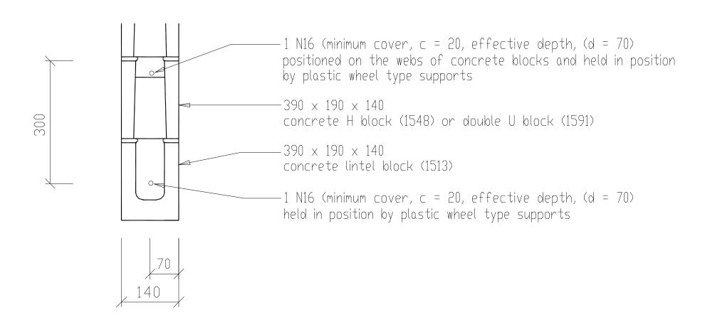
Reinforced Concrete Masonry Lintel Manafactured By Island Block & Paving Scale 1:10
