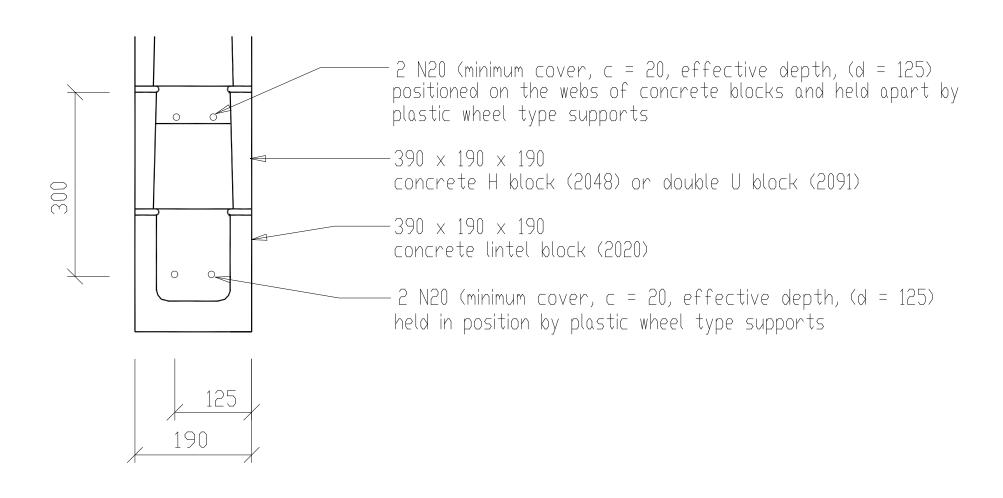
Reinforced Concrete Masonry Lintel Manafactured By Island Block & Paving Scale 1:10
