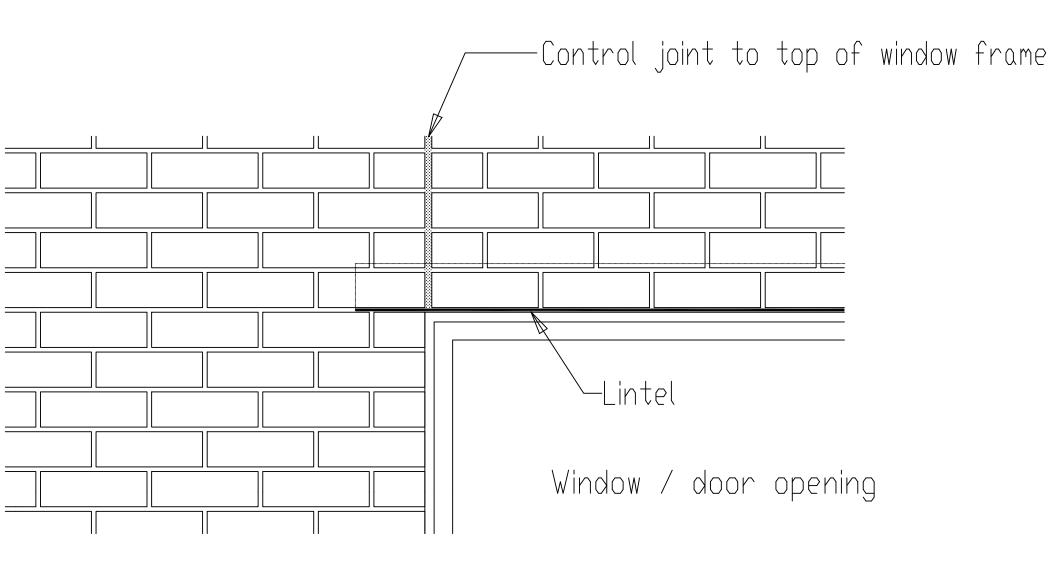
Reinforced Concrete Masonry Manafactured By Island Block & Paving Control Joints at Lintels
