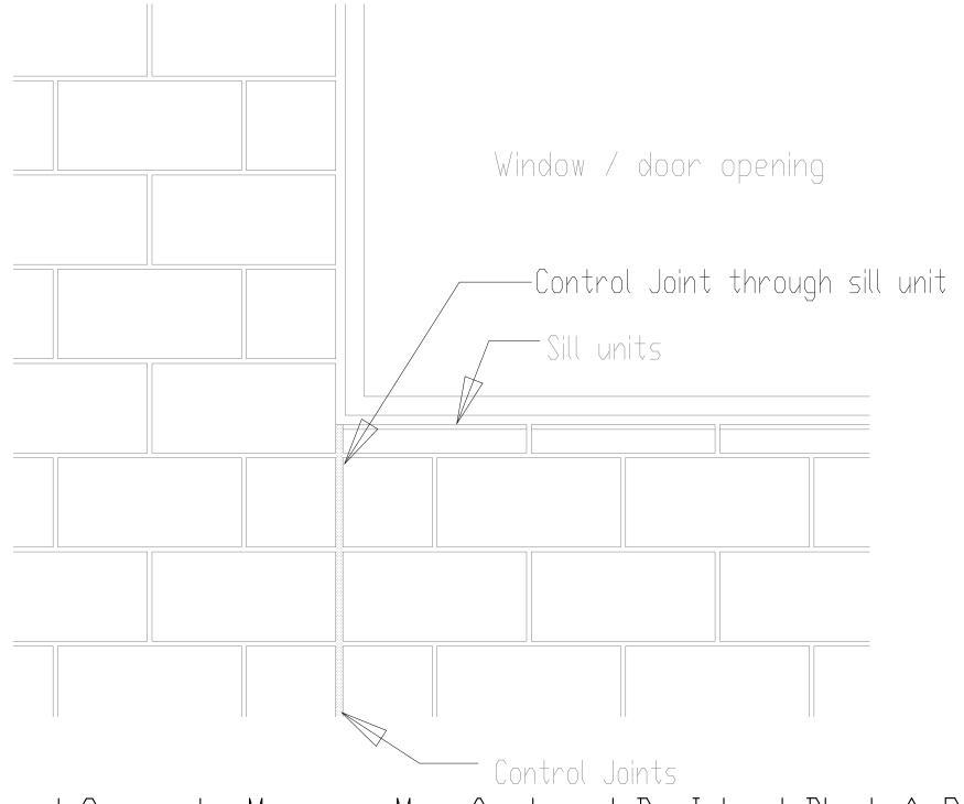
Reinforced Concrete Masonry Manafactured By Island Block & Paving Control Joints at Windows
