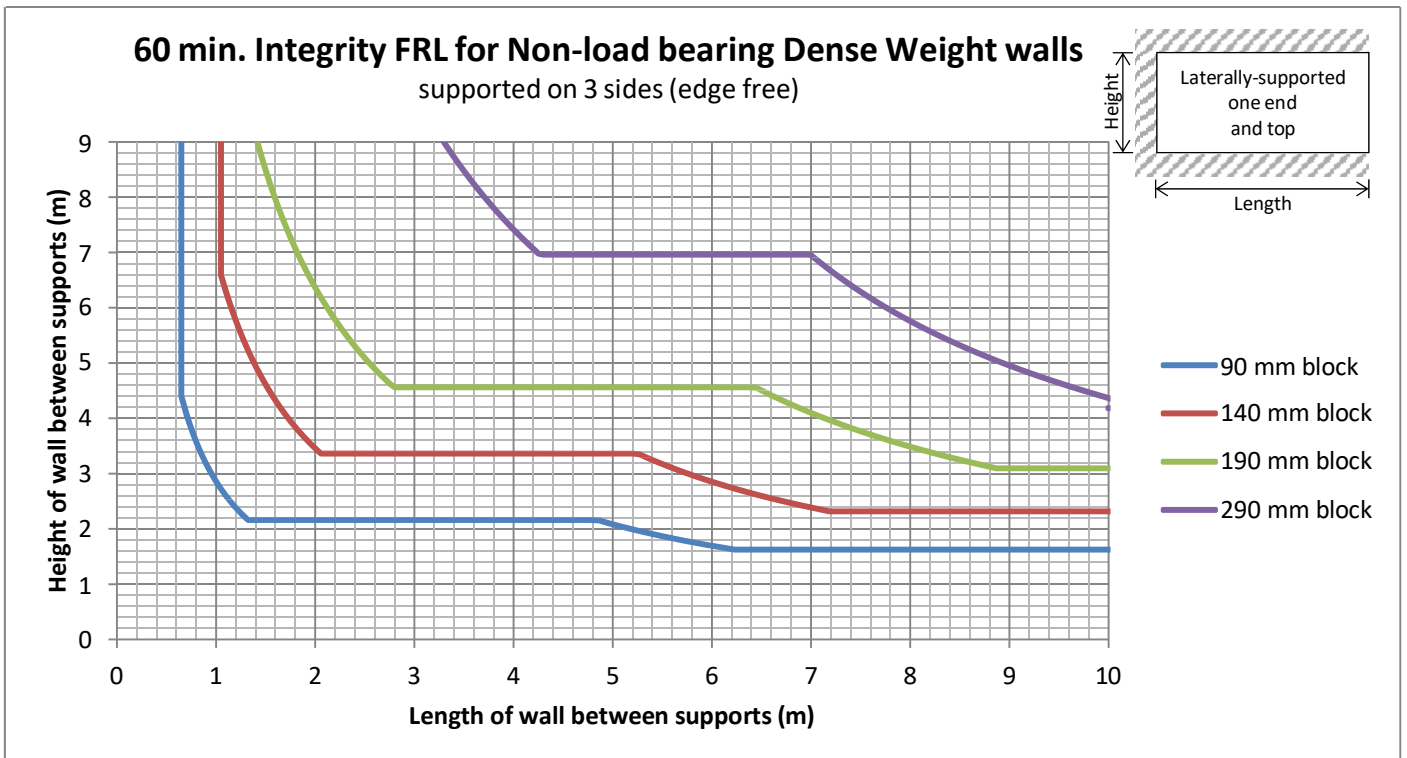
Chart 11 – Dense Weight 60 min. Integrity FRL for walls support on 3 sides (edge free)
